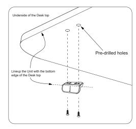
STEP 1 Install the Standard Height Control unit into the pre-drilled holes located on the underside of the Desktop. Before tightening the screws lineup the Unit with the bottom
