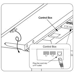
STEP 2 After installing the Standard Height Control unit connect it to the Control Box locaded on the underside of the Desktop between Desk construction beams. Plug the cord into the H1 outlet on the Control Box.
