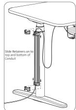
STEP 2. Place cable into the conduit by pushing them down through the center of the conduit.
