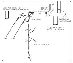
**STEP 3**: Insert Cable Holder onto track flange.
