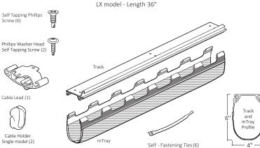
STEP 1: Attach track to underside of work surface.
