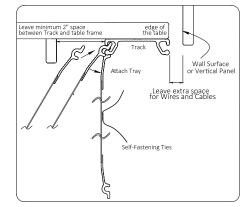
STEP 3: Attach electrical components to the tray.
