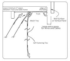
STEP 3: Attach electrical components to the tray.
