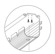
**STEP 2**: Place Cable Holder on the work surface edge • Place the Cable Holder in the desired position along the work surface edge where it can route cables into the cTray.
