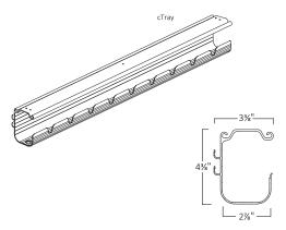
STEP 1: Attach cTray to underside of work surface.
