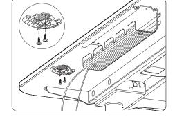
**WARNING**: To be installed on Desk Tops with a minimum thickness of 3/4"
