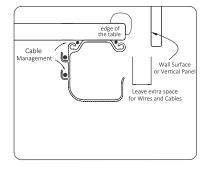
WARNING: To be installed on Desk Tops with a minimum thickness of 3/4"
