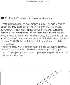
**STEP 2**: Place Cable Holder on the work surface edge • Place the Cable Holder in the desired position along the work surface edge where it can route cables into the cTray.
