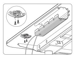
**WARNING**: To be installed on Desk Tops with a minimum thickness of 3/4"
